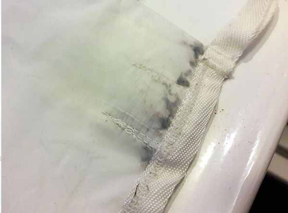
Microfibers collected in the Guppy Friend bag. Photo courtesy Beth Terry ( myplasticfreelife.com )
