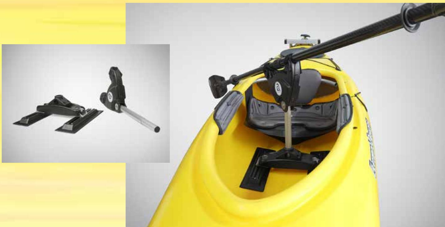
The combination of Creating Ability's Universal Base with this pivoted paddle adaptation allows one-arm control of a kayak. It also provides support to completely remove the weight of the paddle from the paddler's arms. The pivot assembly snaps on to any paddle shaft, and the paddle & pivot assembly lift out of the base for ease of entry and safety in the event of a wet exit.
