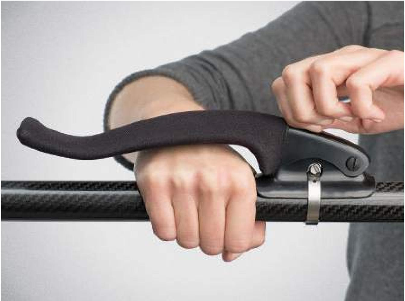
Creating Ability's Back-of-Hand adaptations are designed to relieve the stress of holding the paddle from the fingers and move it to the arms. If the paddler has the ability to grasp the paddle, but lacks endurance or tires easily, this is the correct adaptation. The position is adjustable with a hose clamp, and the arm of the adaptation adjusts up and down easily & quickly with a thumbscrew.
